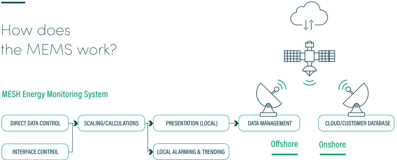
Within a client asset, data is collected from energy producers and consumers. These data points are collected either via MESH installed field instrumentation, or from a client’s existing infrastructure. The data is then displayed through a MESH developed interface.
